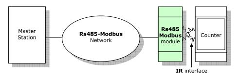
The interface supports both the RTU and the ASCII communication protocols modes and it is configurable for what concern to the transmission parameters (speed, parity, stop bits).
